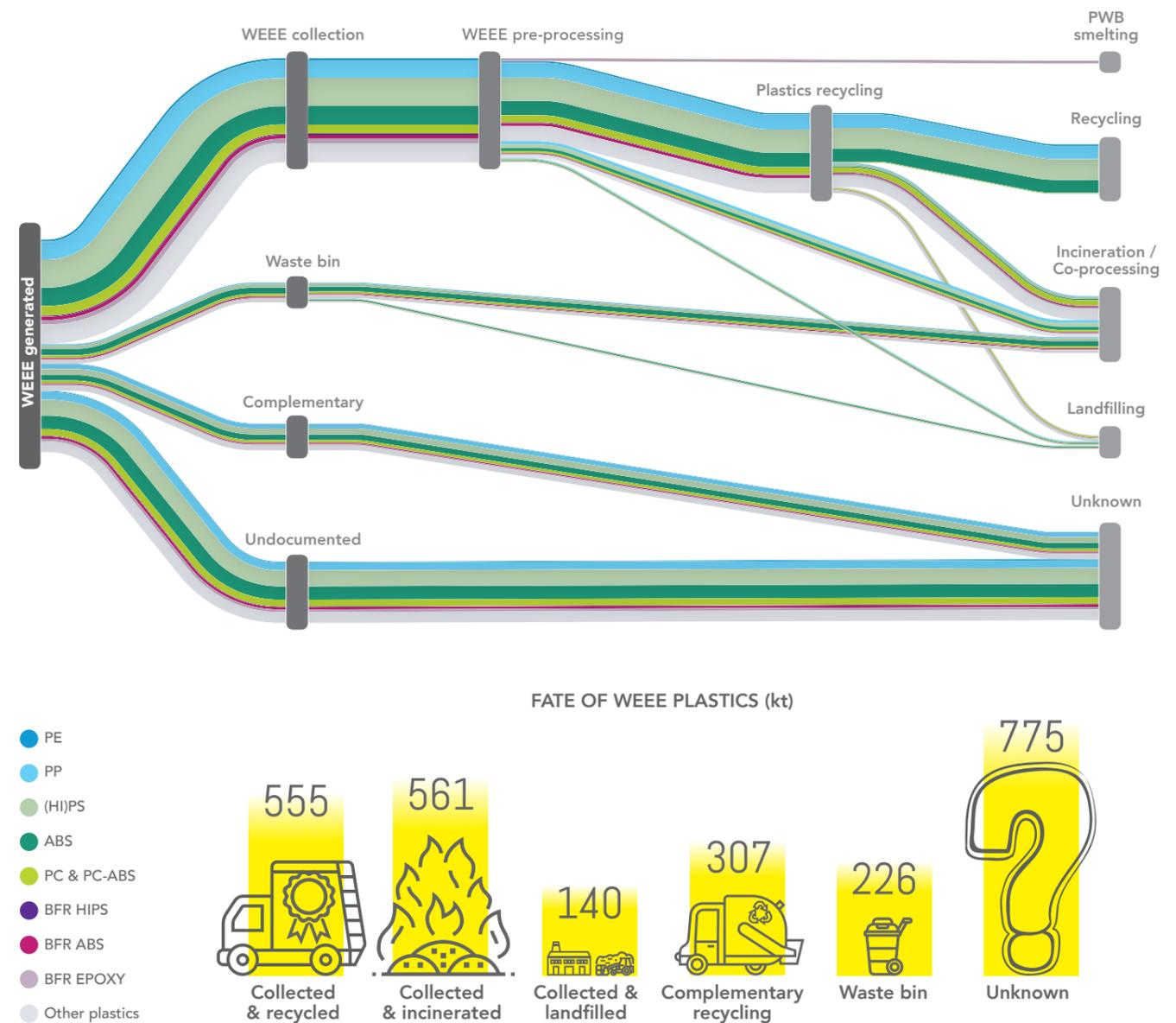
Complementary recycling which refers to the treatment of WEEE mixed with other ferrous or non-ferrous metal scrap, typically under substandard conditions (e.g. lack of depollution) and escaping official WEEE accounting.
