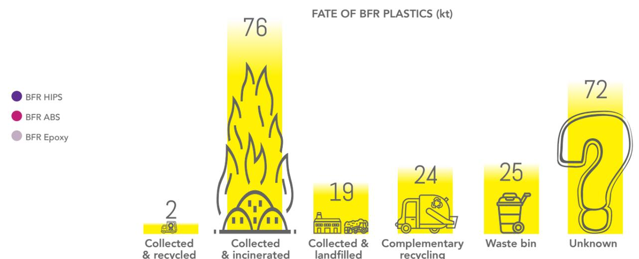
Complementary recycling which refers to the treatment of WEEE mixed with other ferrous or non-ferrous metal scrap, typically under substandard conditions (e.g. lack of depollution) and escaping official WEEE accounting.
