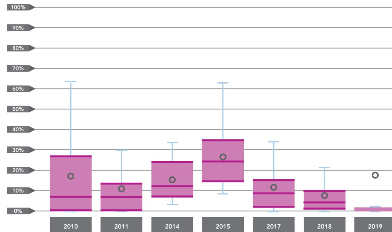
Results show considerable variability in the share of PBDEs relative to the total Br content of samples, with yearly median levels ranging from 0% up to 25%. Despite this variability, a **downwards trend** is clearly visible from 2015 onwards, indicating a phasing out of PBDEs in waste stream. Median levels reached 4% in 2018 (109 samples) and 0% in 2019 (57 samples), meaning that **PBDEs were not found in approximately half of the samples tested in**
