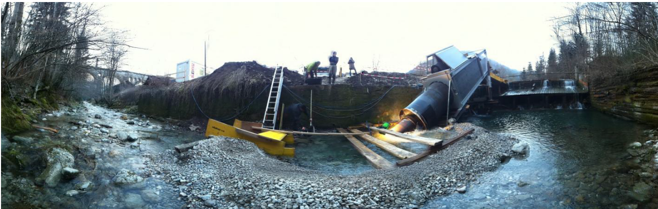
Illustration 1: Panorama picture showing the prototype with tailwater shutoff - dam fill with opened screen at the experiment pool.
