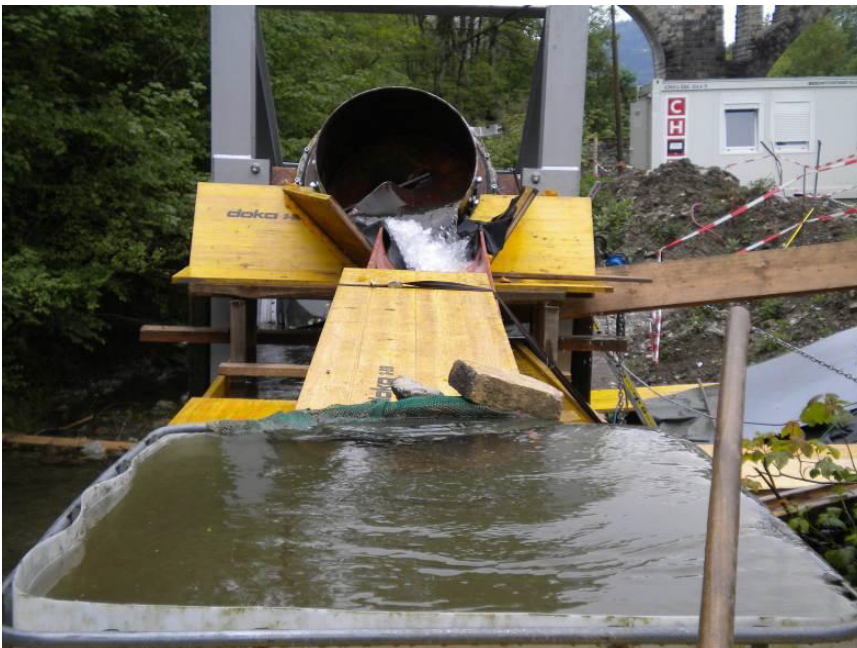
Illustration 2: Fish Migration Aid (FMA) exit with fish slide into the containment basin
